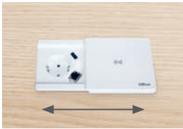
SQ8 electrification module with Qi charging function, sliding cover as inductive charging station, 1 x earthing contact plug, 1 x Ethernet (CAT6RJ45), 1 x USB 3.0, in black or white
